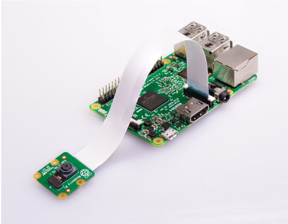
Figure 3: Image of a Pi Camera Connected to Raspberry Pi 3
